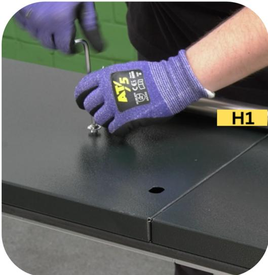
**Screw the two handle screws (H1) into the holes provided.**
