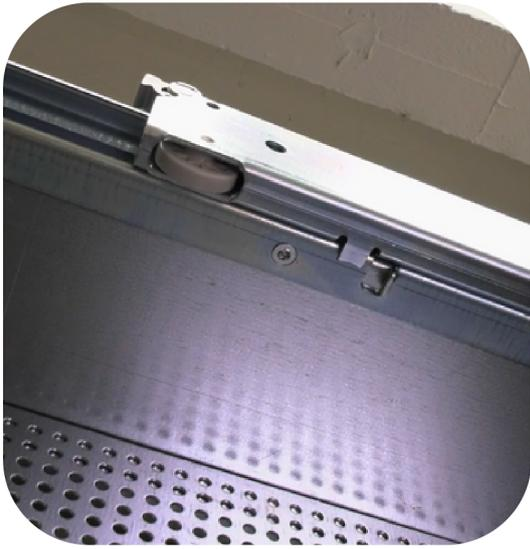
**Check that the rails run correctly in the guide.**
