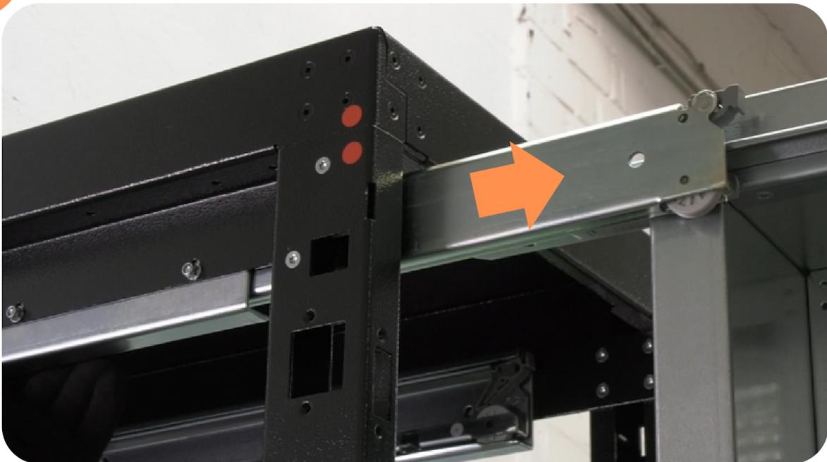
**Pull the guide rails out of the base frame on both sides.**
